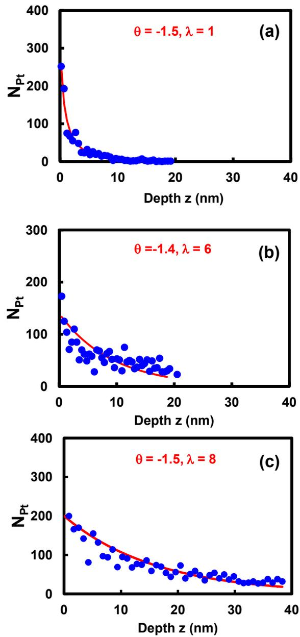
Figure 6: Concentration profiles along the fiber walls (a) on CNF1; (b) on CNF2; (c) on CNF3. the red line is the fitting stretched gaussian function for which  $\theta$  is a relevant parameter (see text)
