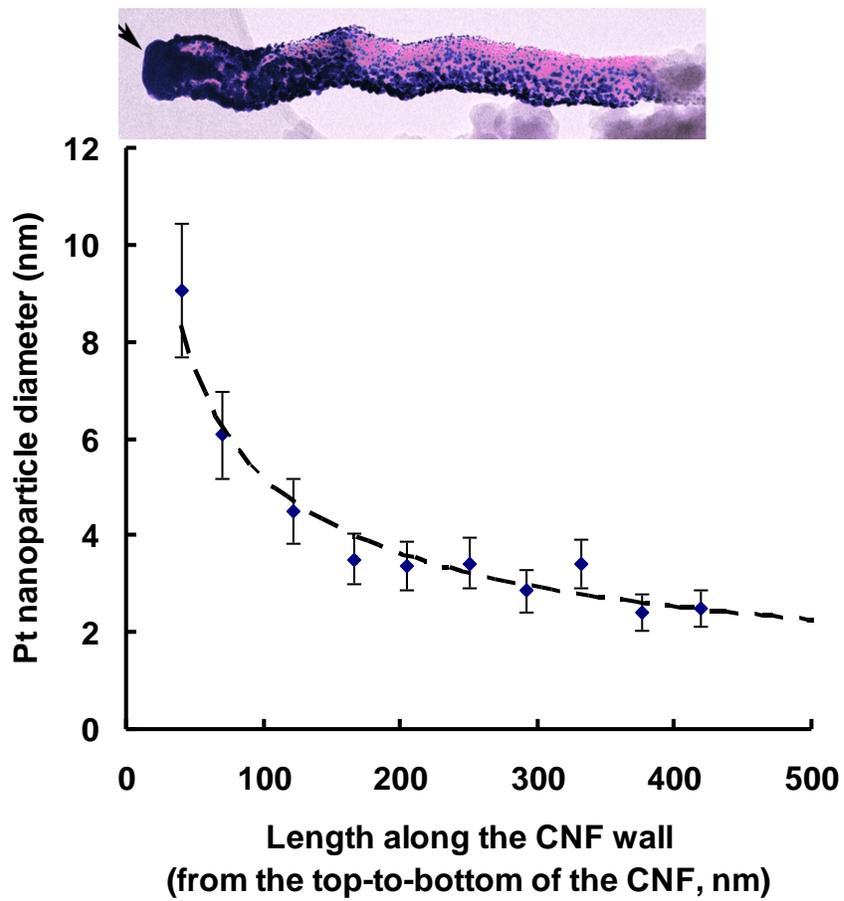
Figure 2: Transmission Electron Microscopy of a Pt "decorated" carbon nanofiber and the corresponding plot of the mean diameter along the CNF length. Pt cluster are dark areas and the arrow on the left indicates the top part of CNF exposed to the Pt flux. The dashed line is for eye guiding
