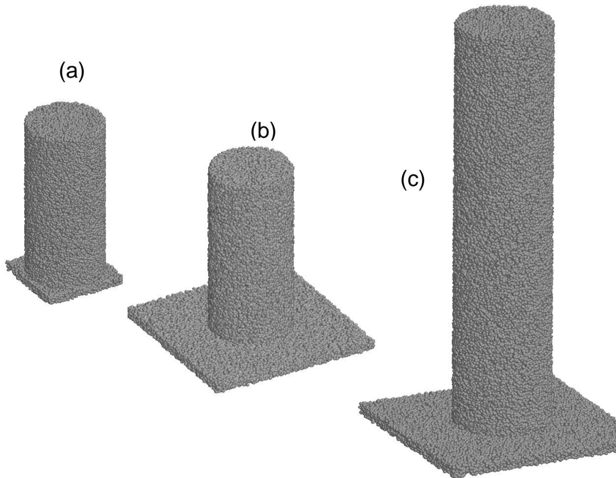
Figure 3: The three model CNF serving as support for Pt deposition. Diameter is 9.2 nm (a) CNF1: substrate is  $10 \times 10 \text{ nm}^2$  and height is 20 nm (b) CNF2: substrate is  $20 \times 20 \text{ nm}^2$  and height is 20 nm (c) CNF3: substrate is  $20 \times 20 \text{ nm}^2$  and height is 40 nm. The spacing (edge to edge distance) between CNF in the equivalent square array, as resulting from periodic boundary conditions is 0.8 nm for CNF1 and 11.8 nm for CNF2 and CNF3
