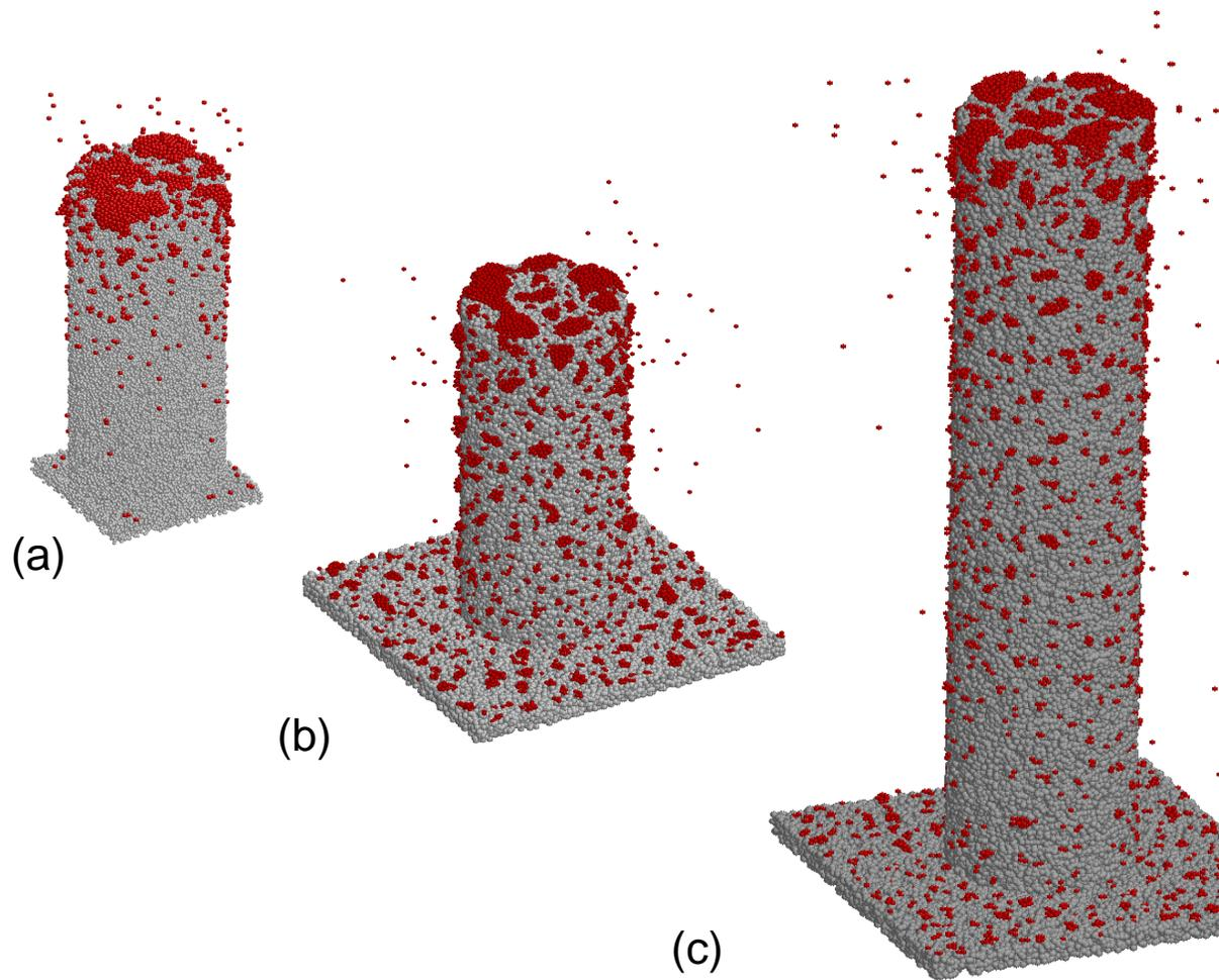
Figure 4: Snapshots of Pt deposited on (a) CNF1 10000 atoms launched, 3149 adsorbed; (b) CNF2: 10000 atoms launched, 5982 adsorbed; (c) CNF3: 10000 atoms launched, 6282 adsorbed
