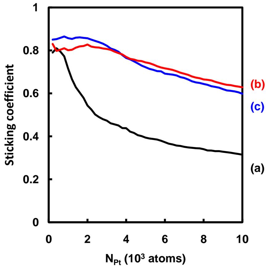
Figure 5: Sticking coefficient evolution vs injected Pt atoms number (a) on CNF1; (b) on CNF2; (c) on CNF3
